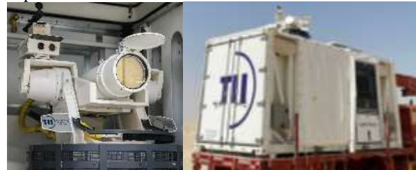
Fig. 1. Photo of LMRL (telescope and container).
