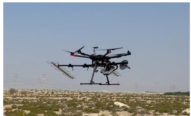
Figure 2. Drone-borne SAR during survey in a rural area in Abu Dhabi, UAE
