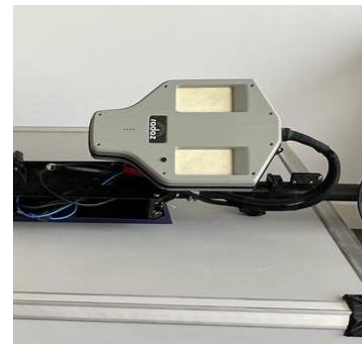
Figure 2. Microwave sensor Cabinet of Explorer RD350.
