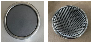
Figure 1 Planar MPG-8 graphite cathode (left). Smooth planar surface with capillaries attached to duralumin substrate (right).
