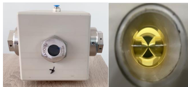
Fig.1 Laser-triggered gas-filled spark gap prototype design.
