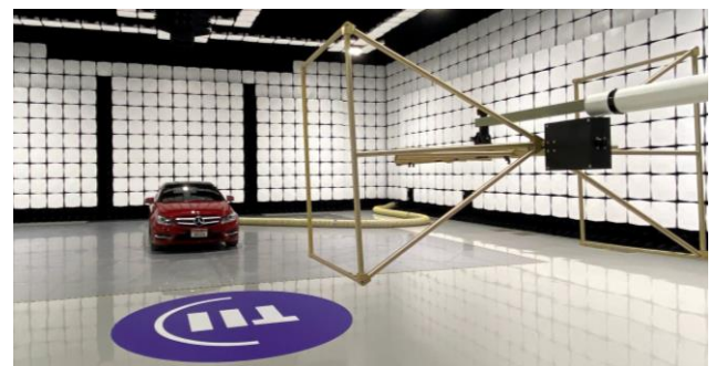
Figure 3. Picture of radiated susceptibility vehicle test.
