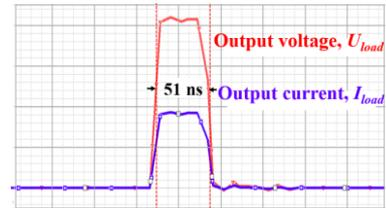
Figure 3. Tesla transformer waveform at rated operations. ( $U_{load}$ : 60 kV/div.,  $I_{load}$ : 20 kA/div., 50 ns/div).
