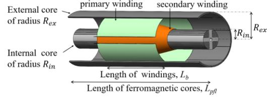
Figure 2. Magnetic core structural diagram of the TT.
