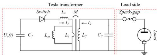
Figure 1. Circuit diagram of open-ferromagnetic cored TT.
